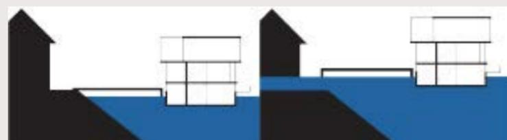
These houses are attached to docks by a mooring system that can move with the tides and sea level rise. The docks connect to artificial islands that contain the utility lines supplying the neighborhood.
