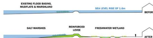
Salt marshes are restored to take in rising saltwater, while freshwater wetlands remediate and absorb excessive stormwater. Together, dual wetlands serve as sponges to absorb water.
