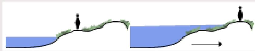
Permanent stop banks are built further back and lower to provide the same protection as higher stop banks close to the river. This creates a more natural river edge, improving habitat for native species. As sea level rises, or storms inundate lower parts of stop banks, human use is pushed to the top.
