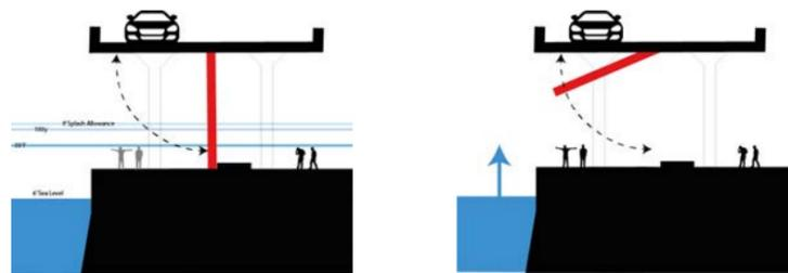
A deployable wall can flip down during storm events to protect from flooding and can transition to a permanent wall to adapt to sea level rise.
