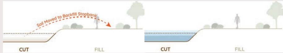
With cut/fill, soil is removed from the area in front of the stopbank and used to build up and widen the stopbanks themselves. Because this strategy 'creates land' by widening the stopbanks, they can become habitable space that can hold trails, infrastructure, and planted areas.
